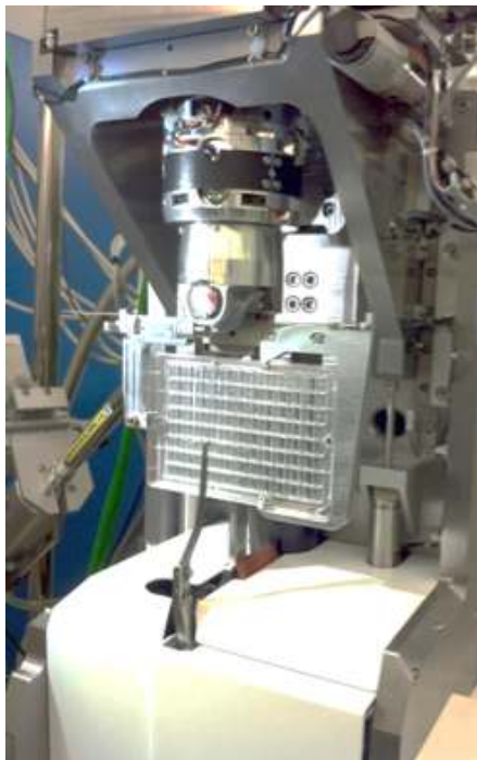
Figure 1. CrystalDirect™ crystallization plate mounted on the MD3 diffractometer for in situ data collection.
