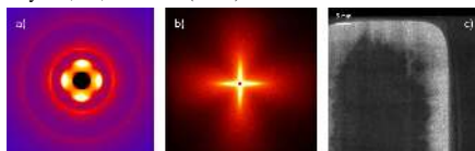
Figure 1. 2D images from WAXS (a), SAXS (b) and X-ray phase contrast imaging (c).
